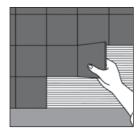
Sweep all debris from underlayment, and vacuum carefully to eliminate dust and dirt.
