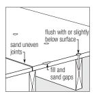
Clean subfloor and leave free of dust, dirt and debris. Ensure that subfloor is completely dry (no more than 12% moisture in subfloor prior to installation). Verify that fasteners are flush with, or slightly below, subfloor surface.
